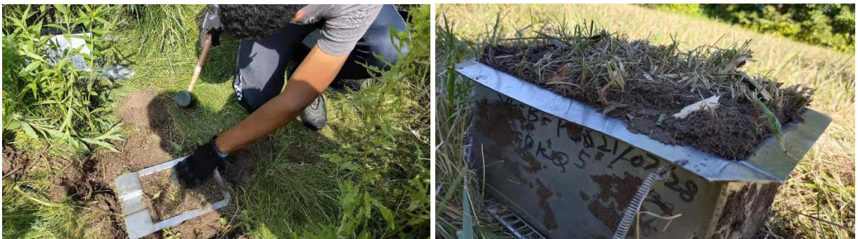
Figure 2. Collecting undisturbed vegetated soil samples using a soil cutter.
